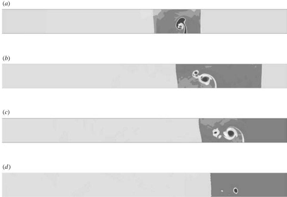
FIGURE 2. Density contours from the direct numerical simulation of the shock interaction with the light gas bubble. Results are shown at times (a) 2.91 ms, (b) 5.24 ms, (c) 7.66 ms and (d) 9.66 ms.
